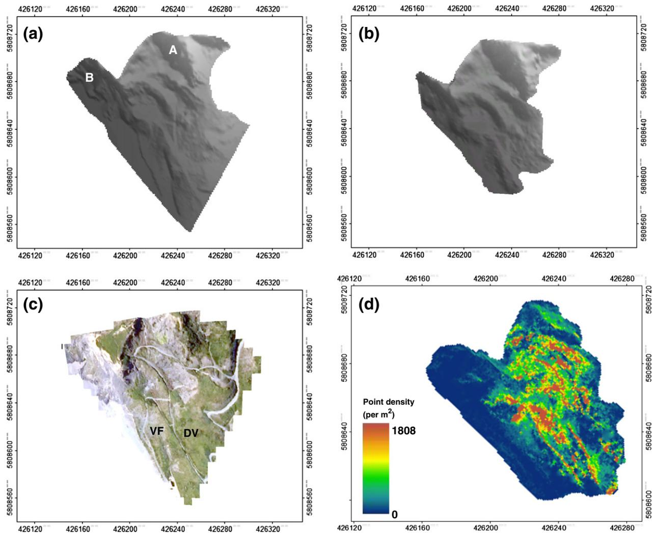
**Fig. 7.** Final interpolated DEMs of Constitution Hill using (a) TLS and (b) SfM data; (c) aerial photograph of the site; and (d) point density map. Panels a and b refer to associated labels in Fig. 5a. VF and DV refer to, respectively, vegetation-free and densely vegetated sub-regions analysed in Fig. 10. Data georeferenced to UTM Zone 30N coordinate system.
