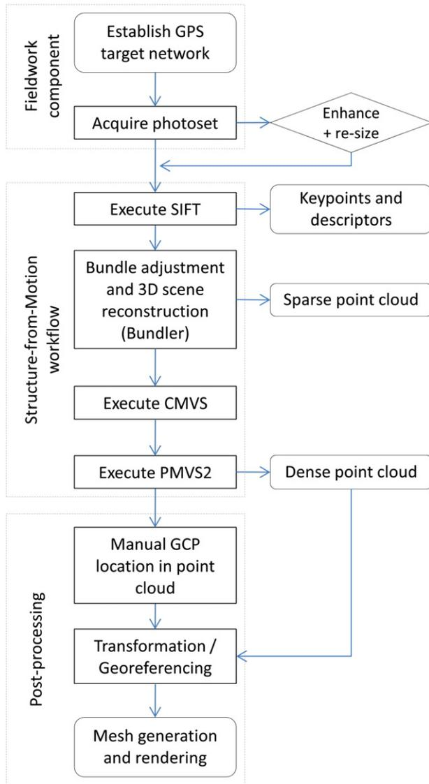
Fig. 3. From photograph to point-cloud: the Structure-from-Motion workflow.
