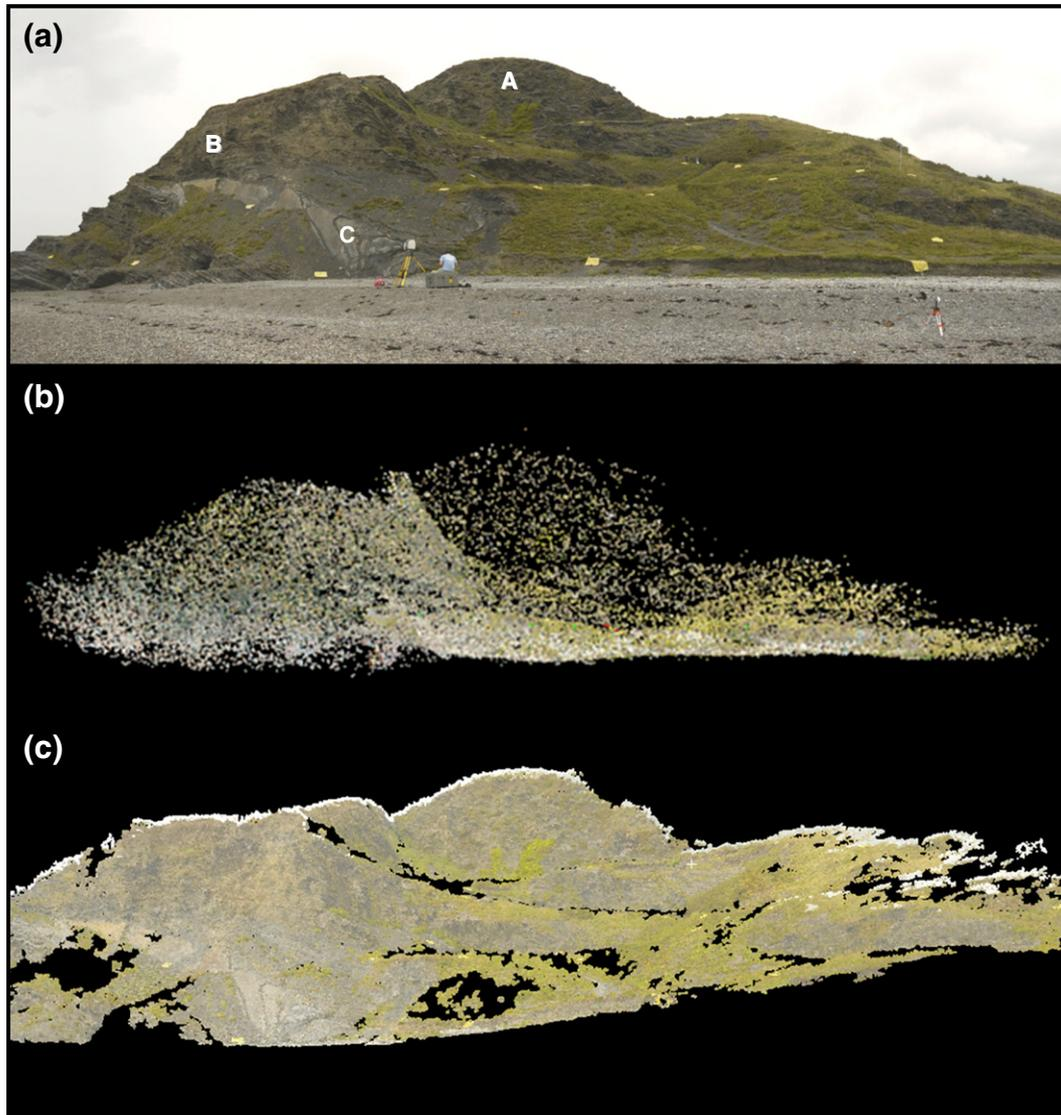
**Fig. 5.** Perspective views of Constitution Hill. (a) Panorama of the survey area with GCPs clearly visible. (See text for description of a and b; c refers to location of Fig. 6), and; (b) sparse and (c) dense point clouds.
