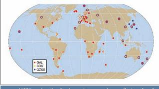
FIGURE 1 MGEX station distribution and supported constellations (as of September 2013)
