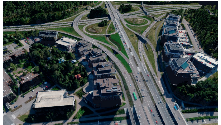
▲ Automatically generated DSM (10cm GSD) from a UAS mission.
