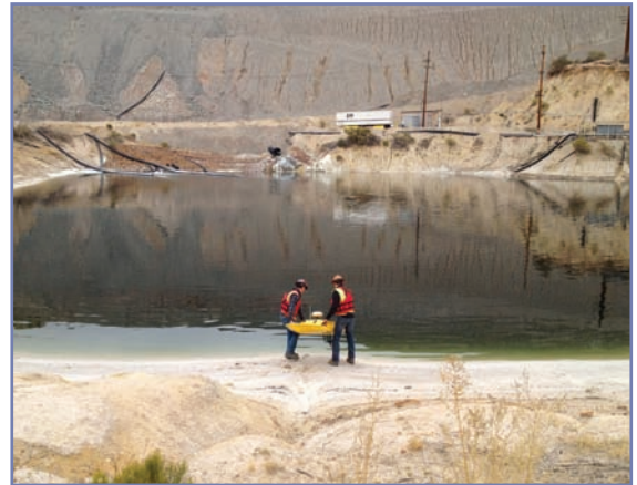
Z-Boat being launched at a leach solution pond
