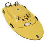
US polar researchers chose the Z-Boat 1800 for a remote bathymetric survey of supraglacial lakes in Greenland. After customization with special reflectance measuring instruments, hydrographic survey grade depth sounder, Trimble RTK GPS, and a stealth black finish, the Z-Boat was used to conduct surveys where a larger boat would have been impossible to transport to the survey site.
