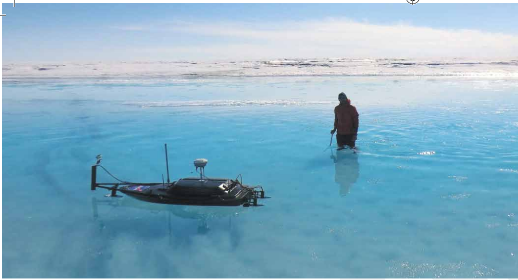
The Z-Boat 1800 used in Greenland was outfitted with a Seafloor Systems SonarMite 200 kHz depth sounder, a SonTek M9 acoustic Doppler current profiler and a Trimble R8 GPS receiver. Below: The Z-Boat is easy to transport to remote locations.
