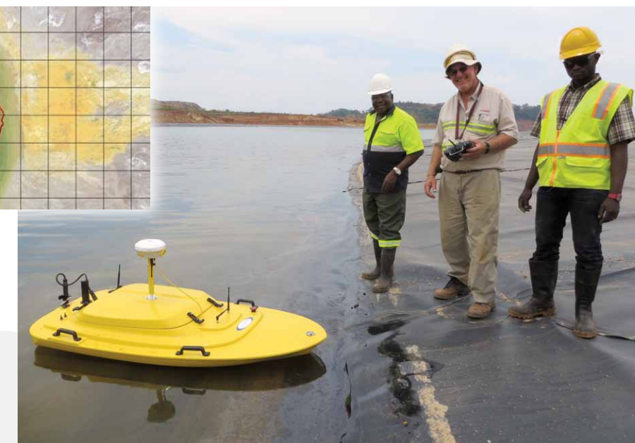
Opposite: U.S. polar scientists in Greenland use a Z-Boat 1800 to conduct studies on supraglacial lakes formed from ice meltwater. Above: Test survey results showing the track of the Z-Boat and associated depths on a portion of a mine tailings dam. Right: The boat is used to collect hydrographic survey data on a remote mine site. Below: Representative data from a bathymetric survey of a mine tailings dam.
